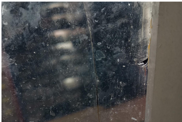
An extreme case of FEP film damage
