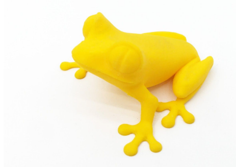
Pict. 20 - 50 microns treefrog is commonly used as a 3D printing benchmark.
